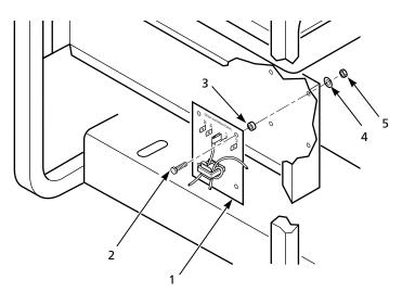
**Control Board Assembly and Mounting**
